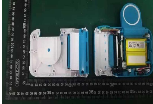
Fig. 5 (phone for children) and Fig 6 (printcam for children) represents toys with a complex system for batteries. It takes time, expertise and the right tools to dismantle and put it back together.
