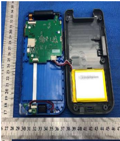
Fig. 5 (phone for children) and Fig 6 (printcam for children) represents toys with a complex system for batteries. It takes time, expertise and the right tools to dismantle and put it back together.
